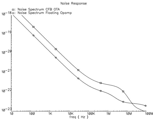
Figure 5: Noise spectra of both circuits.
