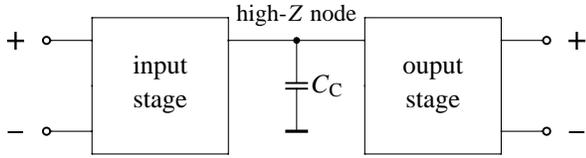
Figure 1: Block diagram of an operational amplifier.
