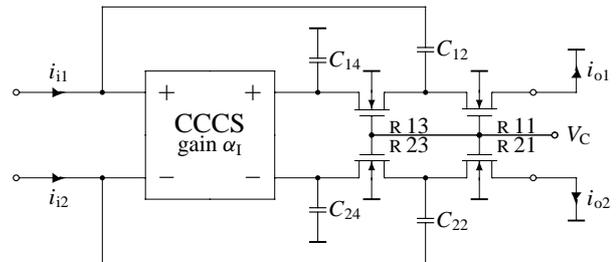
The output of our current amplifier consists of composite transistors, as shown on the right. The cascode transistors are biased with a voltage  $V_m \pm \Delta V$ , where  $V_m$  is the mid-rail voltage. Note that in the process we used, both  $n$ MOS and  $p$ MOS have the same threshold voltage  $|V_{T0}| = 0.85$  V. It can be shown that the  $\Delta V$  that optimises the SNR for a given level of harmonic distortion (e.g.  $-40$  dB) is [7]
