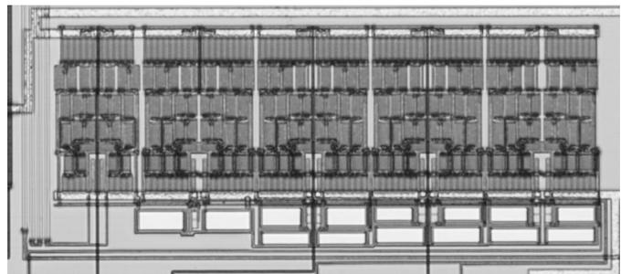
amplifier and a first-order MOSFET-C lowpass filter, and three MOSFET-C SABs with  $(f_p, q_p) = (2.053, 1.13)$ ,  $(1.719, 0.53)$ , and  $(1.825, 0.66)$ , in this order. This filter could, e.g., be used as a pulse equaliser in a  $1 \times$  DVD read channel [11].
